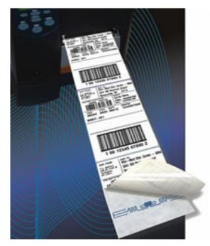
Radio Frequency Identification consists of having an RFID chip embedded within your label stock. The chip is encoded with information based on EPC/RFID requirements, or maybe data dictated by your specific application. The process of encoding this chip involves converting your data to binary, piecing it back together into hex, then encoding it onto the chip. YES, it's complicated.
